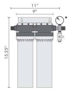
Replacement Filter(s) (2) 310382 - PRO SDS-10 Cartridge
