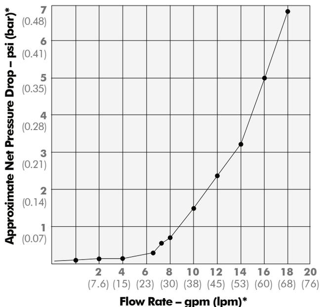
\*Pressure drop and flow rate based on housing without cartridge
