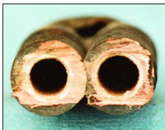
Figure 2. Heat-exchange tubes showing (from top) blockage by scale buildup, tubes cracked due to corrosion caused by repeated acid cleaning, and clean tubes after water treatment.
